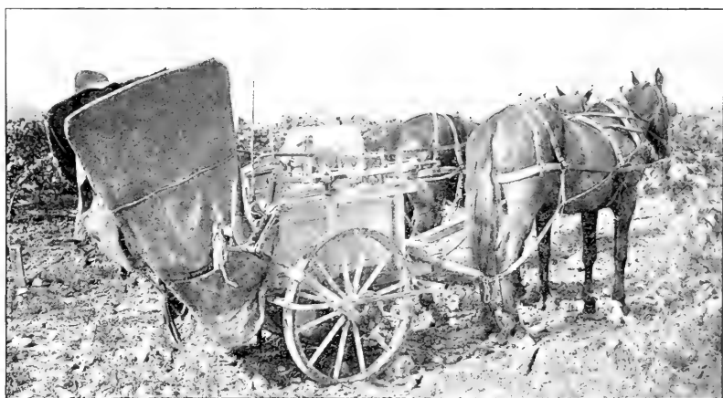
FIG. 27.—A vineyard sprayer combining horse-power and compressed-air power. Note the effective, home-made screen to keep the spray from the driver.
